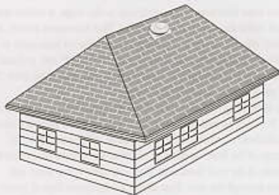
Figure 7-25: Power fans are used to move large volumes of air — a good option for hard-to-vent hip roofs.
