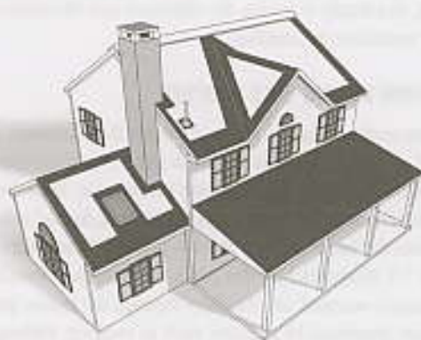
Figure 7-6: The dark shaded areas are the places that WinterGuard helps protect from the melting water coming off the ice dam.
