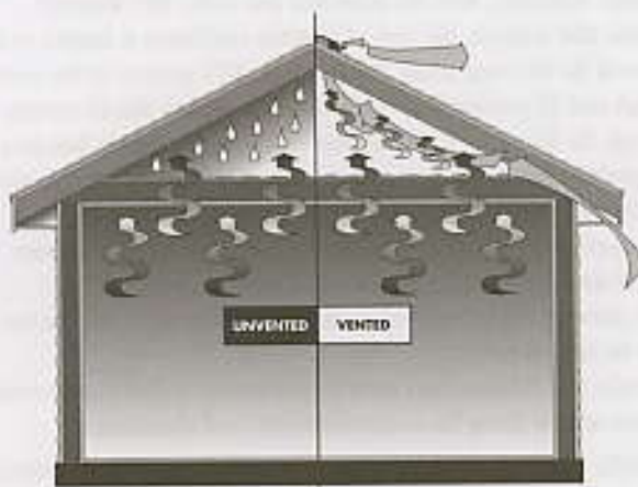
Figure 7-8: Attic ventilated by thermal effect.
