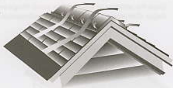
Figure 7-23: An externally baffled vent “pulls” air from the attic through both side of the vent.
