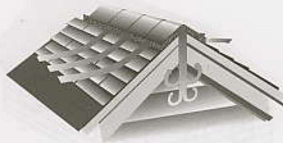
Figure 7-22: A roll vent with an internal baffle, or without any baffle at all, does not “pull” air from the attic through both sides of the vent.
