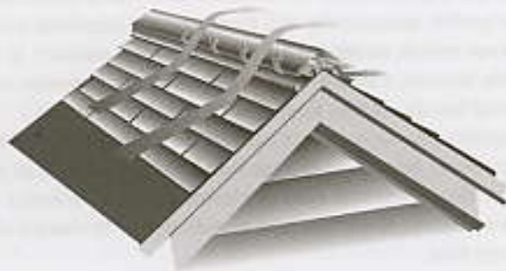
Figure 7-20: A baffled FilterVent® creates an area of low pressure on both sides of the ridge vent. It literally lifts air out of the attic through both sides of the vent.
