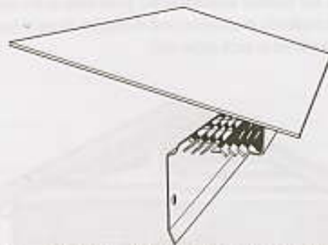
Figure 7-15A: For soffitless applications vented drip edge combines a drip edge with intake louvers.
