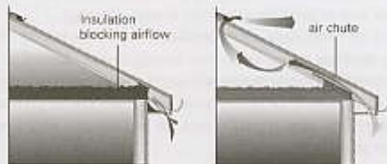
Figure 7-10: (Left) Insulation should not be installed over the soffit/underside intake area or proper inflow to the attic will be impeded. (Right) An unblocked vent allows a passage for air to move through the attic.
