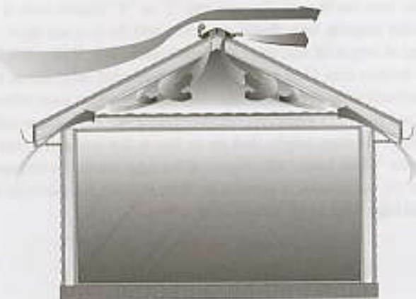
Figure 7-7: Thermal Flow (effect whereby cooler air falls, warmer air rises) and Natural Flow (effect due to wind) come together to ventilate an attic.
