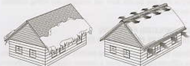
Figure 7-4: (Left) Ice dams, besides being unsightly, are destructive. (Right) Vented attic with even snow distribution is much more desirable.
