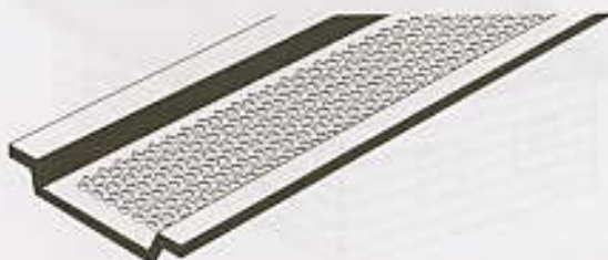
Figure 7-14: A continuous soffit vent takes in outside air and is located on the underside of the eave.
