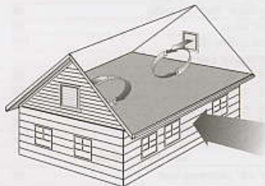
Figure 7-18: With wind blowing perpendicular to the ridge, the louvers act as both intake and exhaust vents.
