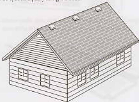
Figure 7-16: A roof louver is an exhaust vent located near the ridge.
