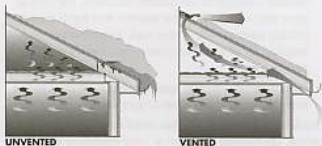
Figure 7-3: Unvented: Heat entering attic from the home melts the snow on the roof and forms destructive ice dams. Vented: Heat is vented out of the attic creating a cold roof.
